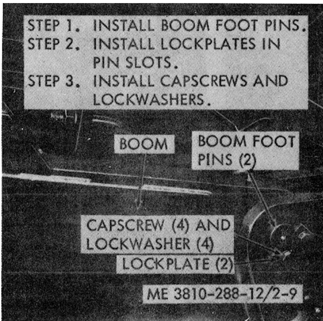
Figure 2-9. Installing boom foot pins.
